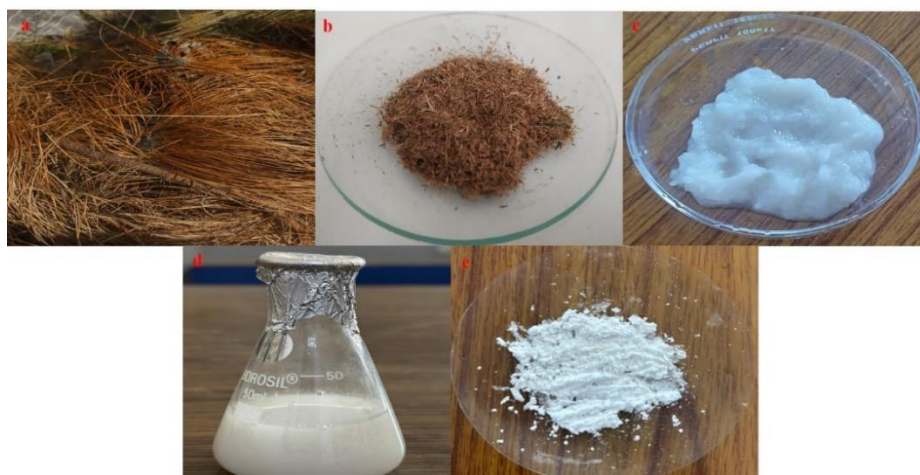
Fig. 3: Physical aspect of the (a) raw dried pinus needles (b) Grinded pinus needles (c) Extracted cellulose (d) Nanocellulose suspension (e) Cellulose nanocrystal powder
