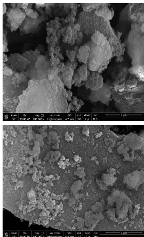
**Fig. 4:** SEM micrograph of as-groomed (T1) and annealed sample (T2) at 900°C.
