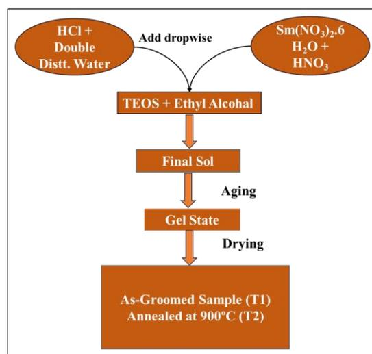
**Fig. 1:** Sol-gel method for formulation of samarium doped silica nanopowder.
