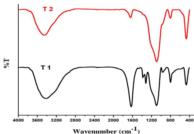
**Fig. 3:** FTIR Spectrum of as-groomed (T1) and annealed sample (T2) at 900°C.
