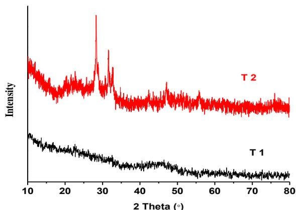
**Fig. 2:** XRD patterns of as-groomed (T1) and annealed sample (T2) at 900°C.
