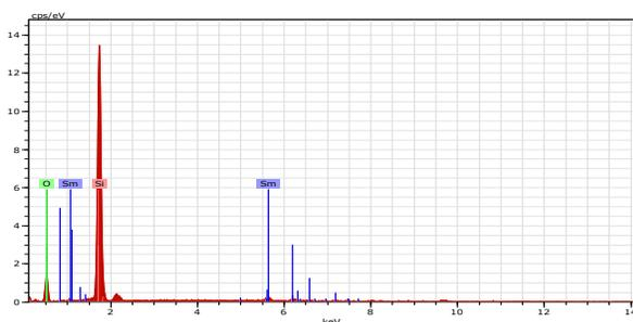
**Fig. 5:** EDX (Energy dispersive X-ray) spectrum of annealed sample T2.
