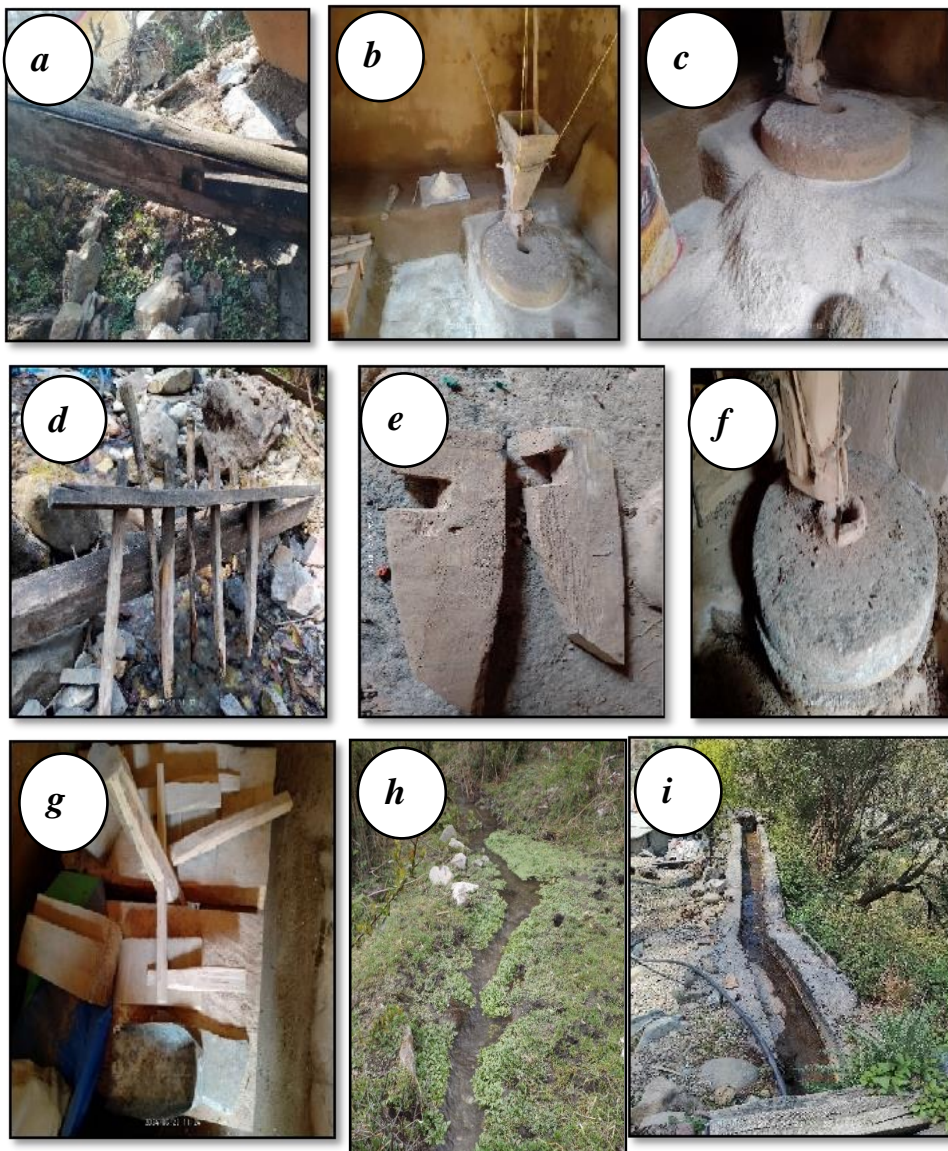
Fig. 4 Upper ground Parts of Indigenous Flour Mill (Gharat)
